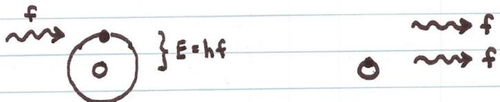
Cloned photon has same frequency, phase, direction of incident photon
